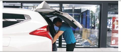
Anti-pinch function: 1. Anti-clamping: When the obstacle is under the tailgate closed, when the tailgate is closed, When you encounter an obstacle, you will bounce back in the opposite direction 2. Door collision avoidance: When the obstacle is behind the tailgate Obstacles will bounce back in the opposite direction
