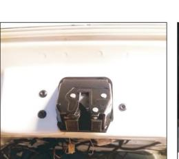
25. Remove the original car door lock, install our electric suction, use the original car screws
