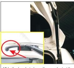
12.In the bracket above the punch strut line through the hole to the tail door cover
