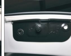
3. Install the special upper right bracket of our company. As shown in the picture, the original vehicle ball head uses our balance screw fixing bracket.
