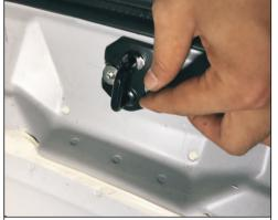
24. Install our special lock, fixed with the original car screws
