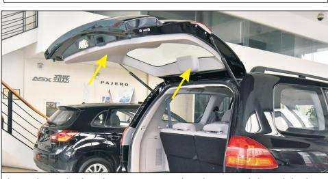
1. as shown in the picture, remove the plaque and the original car electric pole.
