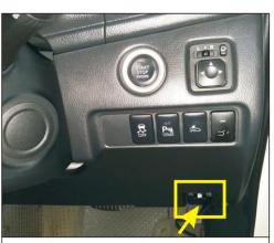
20. OBD insertion below switch before main driving
