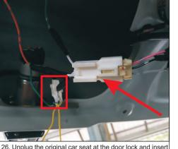
26. Unplug the original car seat at the door lock and insert the three-way adapter socket of our company. The white socket of the electric lock and the socket of the three-way wiring harness are inserted.
