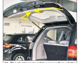
electric pole harness wiring
