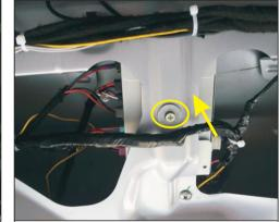
31. Control box installation position, with our screws, gaskets, mesons
